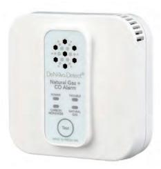
As such, natural gas alarms are critical if an occupant is not able to smell natural gas or if small children or elderly occupants are present, which creates a higher risk for a gas stove burner to be left on without a flame. These life saving devices work by sensing natural gas and sounding an alarm before the gas reaches the explosive range to keep you safe.
